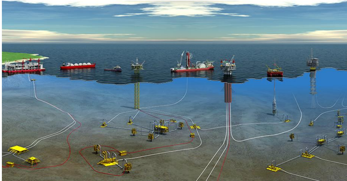
Figure 16. Typical subsea field development options – tied back to a host facility
