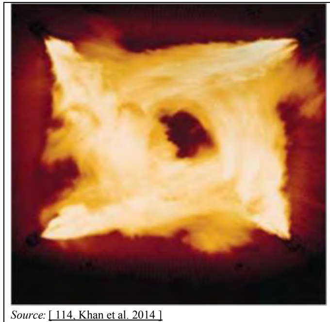
Figure 2.2: Tangential-fired combustion chamber
