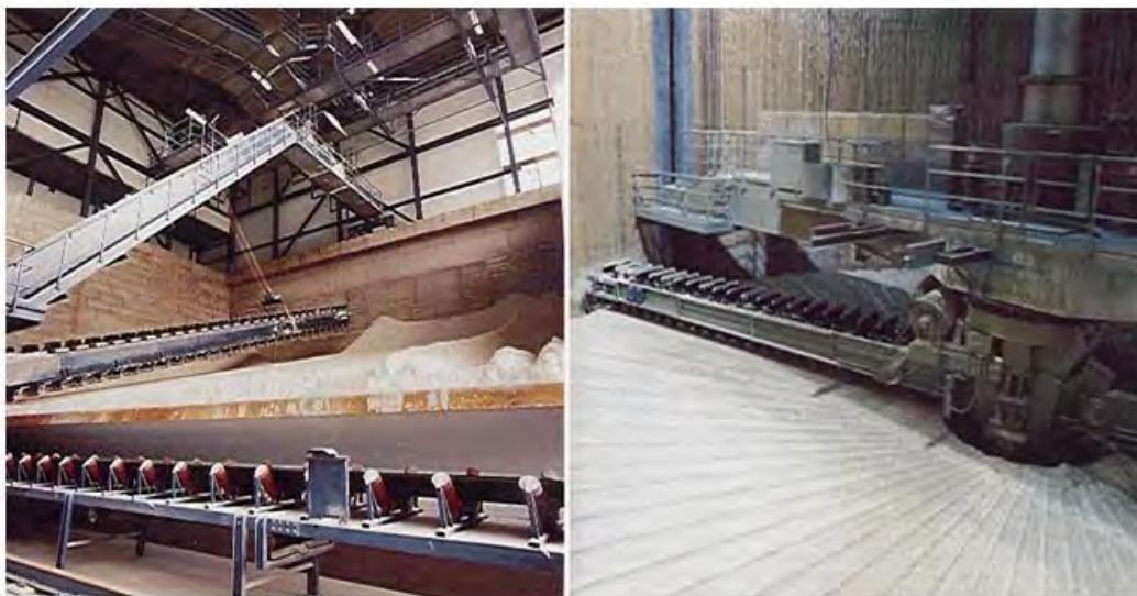
Figure 5.8: Closed gypsum storage facilities
