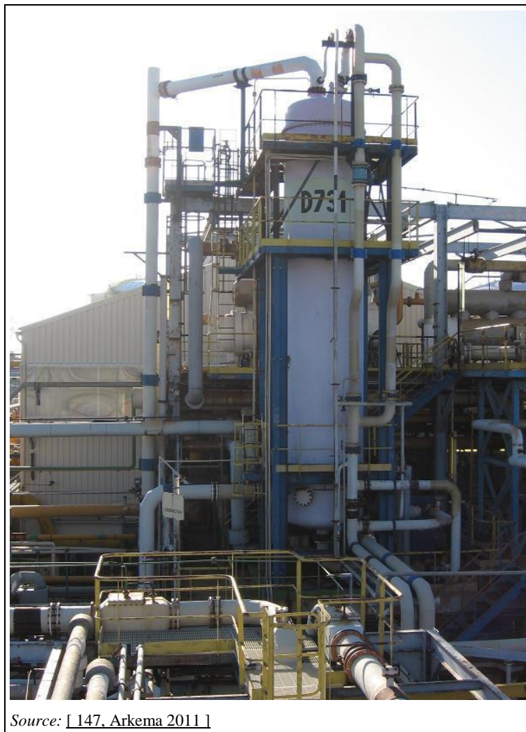
Figure 2.18: View of a chlorine absorption unit
