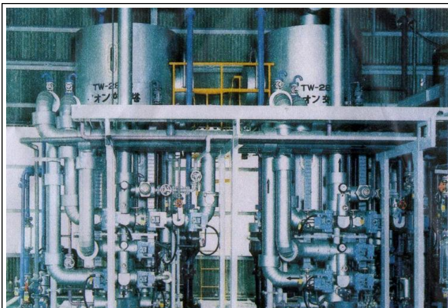
Figure 2.17: View of chelate resin towers in a secondary brine purification system
